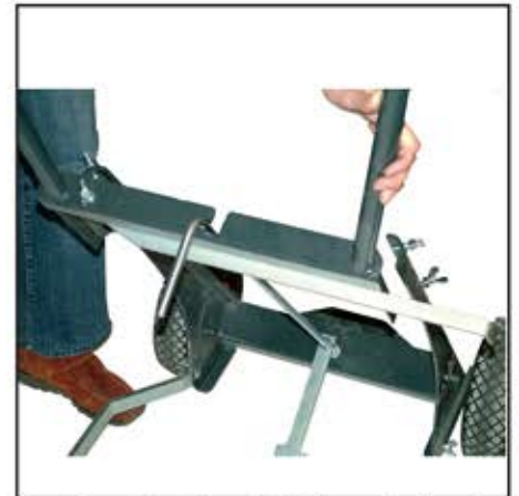
Tighten the upper part with the 4 wing nuts. Pay attention that the axle bar is correctly fitted through the cuttings.
