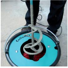
Place the dirty mixing paddle between the brushes, make the mixer rotate slowly until it is completely immersed.
