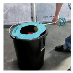
The two retaining projections slide out of the mountings, the cover with the brushes can be taken out.
