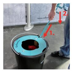
To open the bucket, you can use the shaft of the mixing paddle or another suitable tool. Stick the tool into the opening provided and push up the cover with the brushes.
