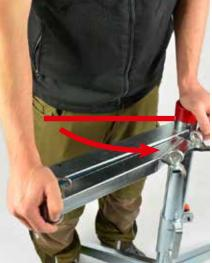
Hold the round pipe in the depressed position and swivel the square pipe to the side. When the release is actuated, the spring force will press the swivel arm upwards.
