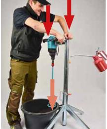
For mixing: push the machine into the material and move to all sides. To support while starting, press the tube with your second hand downwards to get the mixer lowered easily; grease the tube slightly
