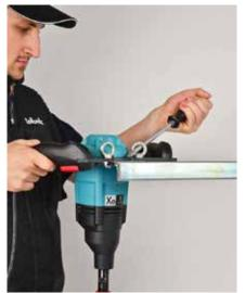
Secure the mixer firmly with the screws; if necessary use a tool to tighten the screws
